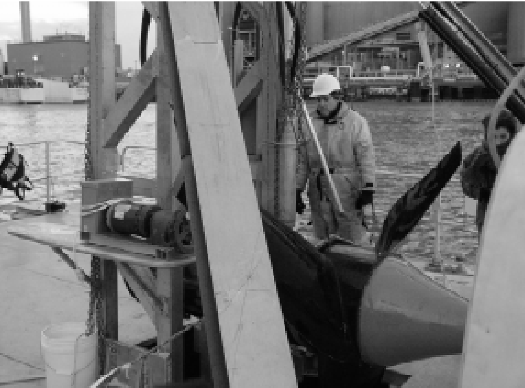
On the turbine evaluation vessel, the crew raises and lowers this ten-foot-diameter propeller with tidal cycles to check it for damage, while...
