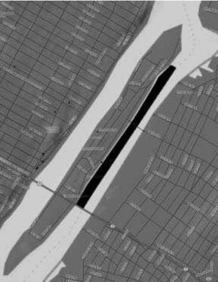
Map segment shows the underwater turbine field envisioned in the Verdant Power plan. The units are to be 8-12 feet below the surface.
